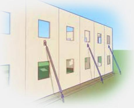
**Freestanding Bracing** is used when wall panels are erected prior to the structural steel system. A temporary brace is installed diagonally from the wall panel (either interior or exterior) and secured to a “deadman” anchor. This hold the panels in place until the steel arrives.
